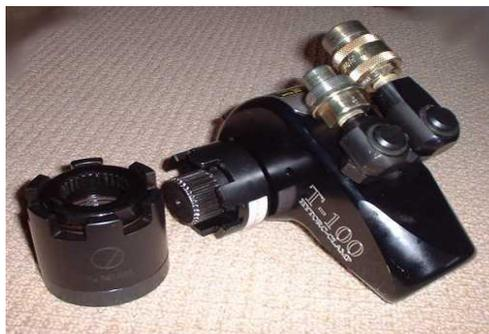
The Hytorc Clamp with the JETYD T-100 load-stretching tool alongside. Note the splined drive assembly. The Hytorc Clamp is also available in a limited clearance version, worked from the side.
